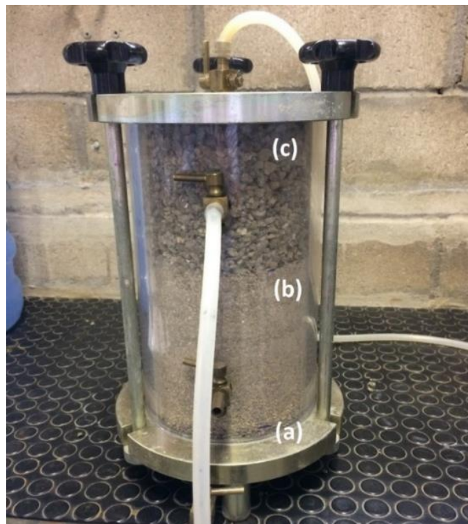
Figura 11 – Permeômetro compreendendo as camadas (C), (B) e (A)
